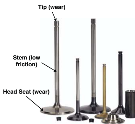
Figure 4. Most valves have different coatings on different parts. Decreasing friction is critical on the stem, while wear resistance is the primary concern for the head. The photo also shows valve spring retainers, valve locks, and piston wrist pins, all of which are also coated. Images courtesy of Xceldyne and CV Products.
